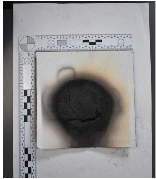
Figure 11: V; 5VA; Representative image at flame application
